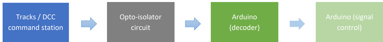
Figure 13: Decoder connection schematics
